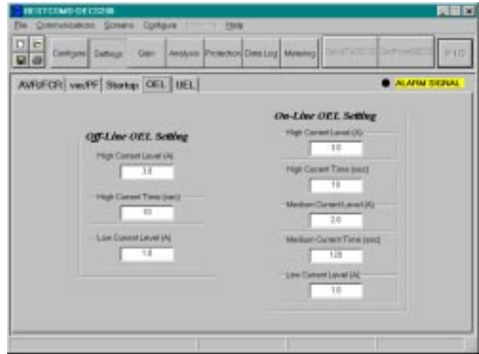
Figure 3: BESTCOMS settings screens allow the user to type in settings values for fast and easy commissioning.
